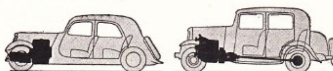
Front wheel traction permits of a perfectly flat undershield
