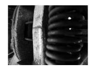
Handbrake Spring for Pads
